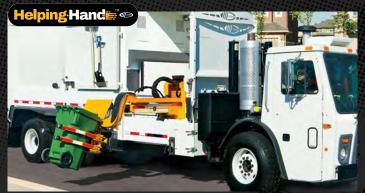
Collect from the comfort of the cab while still having the option to pick up extra items left on residential routes. The Helping-Hand™ arm has a pivot point that provides a minimal swing-out motion. making it ideal for dumping in narrow spaces and alleys. It can extend up to 10 feet and lift up to 400 pounds when fully extended. By being located inside the hopper, the Helping Hand eliminates the need to compensate for torsion stress, reducing wear and tear on the arm's components.
