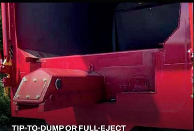
The Full-Eject system with T-Track Guide extends the lifespan of packer and wear components. A single cylinder handles both packing and full ejection.
