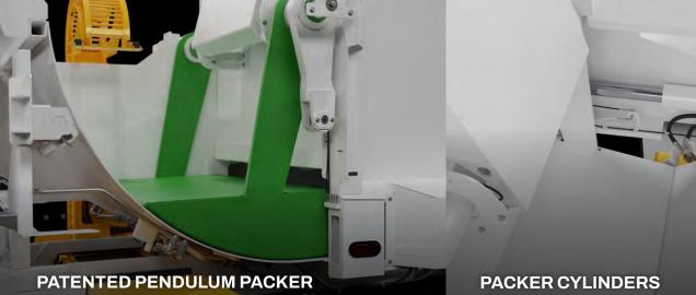
The Patented Pendulum Packer is low maintenance with no wear tracks or follower panel. Ideal for organics and solid waste with its sealed hopper.
