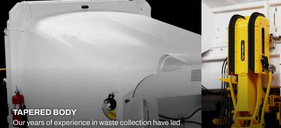
Our years of experience in waste collection have led us to create a proven, tapered body design. The rounded and tapered shape of the body sides and roof increases the compaction ratio by retaining the majority of the material at the back of the body.
