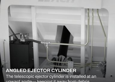
upward angle—keeping it away from debris, and directing compaction forces away from the body floor and towards its front mount location.
