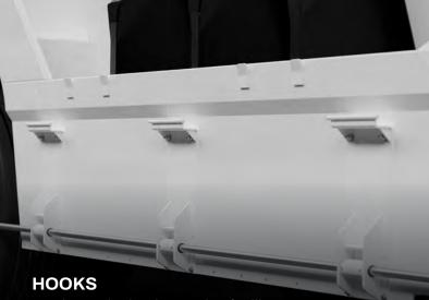
Hooks on the bucket's edge facilitate easy sorting and handling of recycling boxes.
